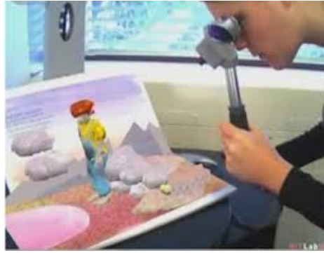
Figure 20. A user is viewing the MagicBook using a hand-held video see through display.
